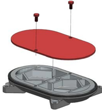
Fig. 10.3.1.1 “No hole” cover wear plate installation
