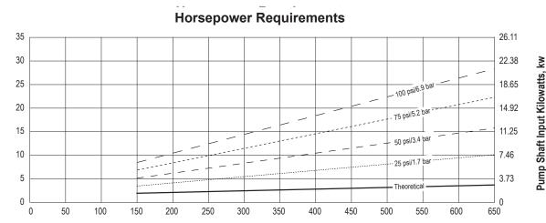
Pump Speed, rpm
